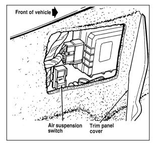
The air suspension switch — located in the trunk
